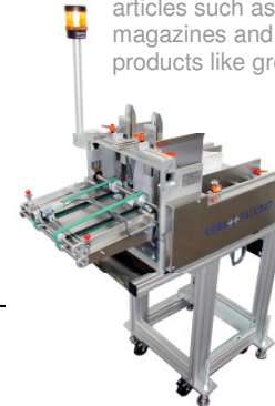
LSA sliding feeder for the separation of thick brochures and catalogues.
